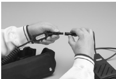
Figure 8: AirBelt Battery Charging
